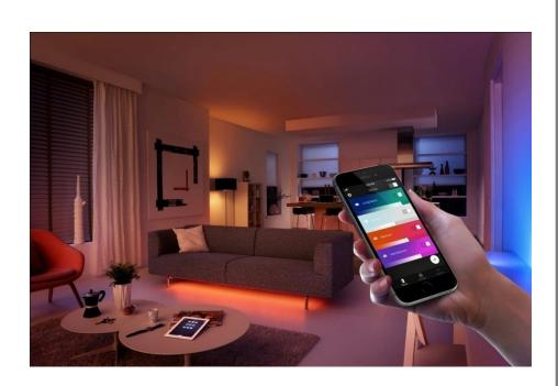
Wireless lighting contain various LED specially chosen to produce wide range of intensities and over 16 million colours; Wirelessly controlled by mobile application
